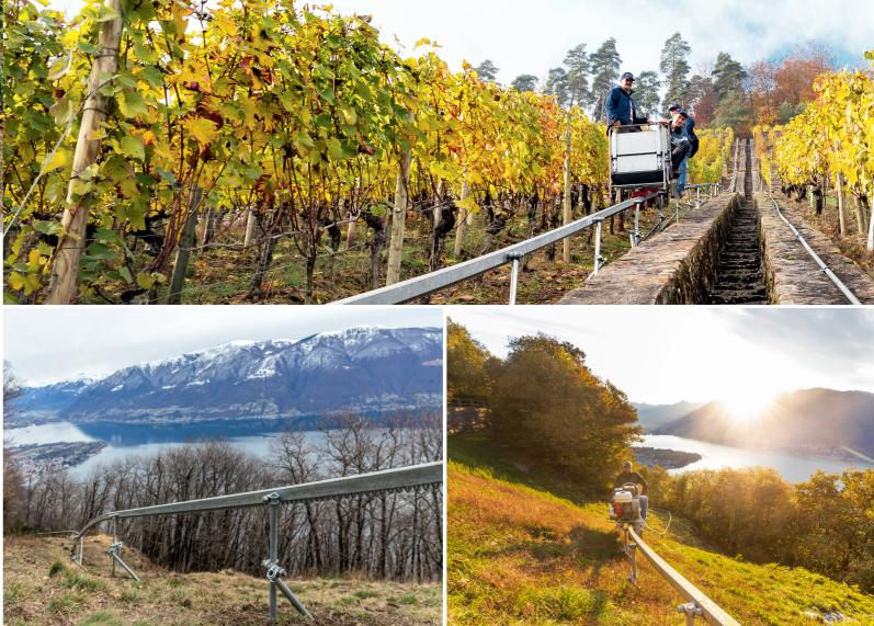
The track consists of the running rail and the sup- life. The use of different switch rails makes it possible to connect several lines together. Bridge elelong rails with welded splines as well as the supments allow the crossing of challenging sections of port material are hot-dip galvanized to protect them terrain according to the customer's needs and local
