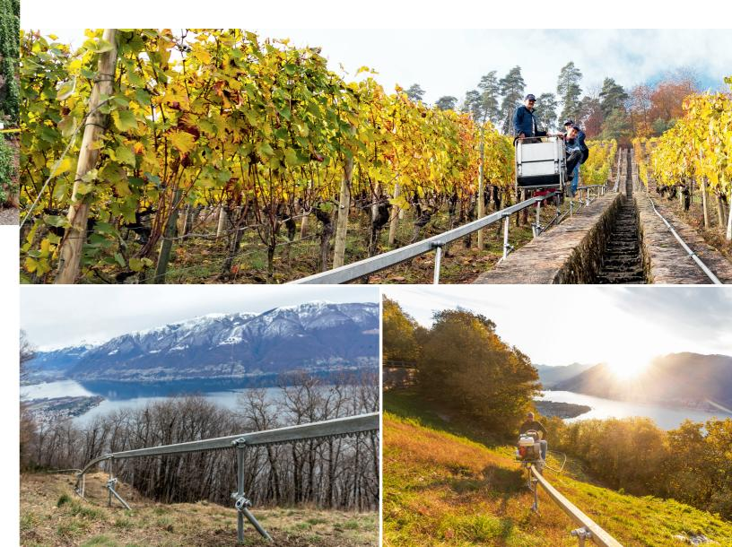
ge extend be adapted to the terrain. The Monorack higher norm pipe-supports. Boarding, deboarding, can easily handle gradients up to 100% as well as loading and unloading are possible anywhere with horizontal and vertical curves with a radius of up to the appropriate track layout.
