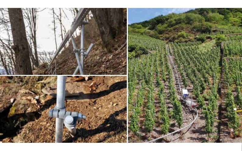
The route of a Monorack installation can to a large extend be adapted to the terrain. The Monorack can easily handle gradients up to 100% as well as horizontal and vertical curves with a radius of up to four metres. High walls can be surmounted by using higher norm pipe-supports. Boarding, deboarding, loading and unloading are possible anywhere with the appropriate track layout.
